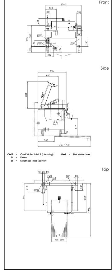
ProThermetic Sprint Electric Tilting Pressure Braising Pan, 90lt Hygienic Profile, Freestanding with CTS The company reserves the right to make modifications to the products without prior notice. All information correct at time of printing.
